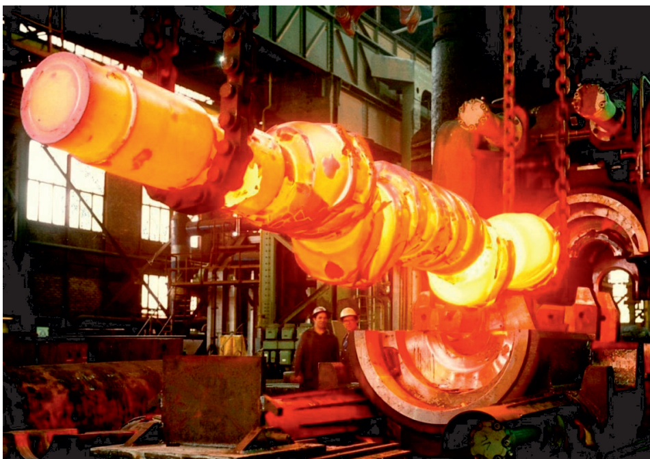
Figure 2.20. Forging of crankshafts using the TR method
